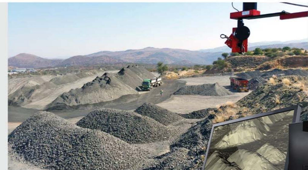
ABOVE: The ARTEMIS® 300 series scanner applied to OPEN AIR STOCK PILES.
