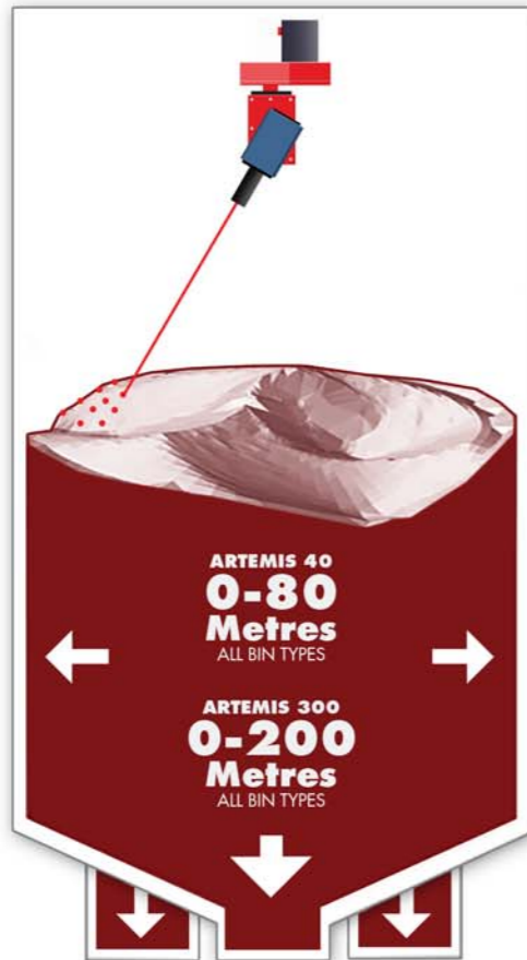
ABOVE & LEFT: The ARTEMIS® 40 series scanner applied inside STORAGE BINS, BUNKERS & FLAT WAREHOUSES.
